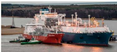
2<sup>nd</sup> January 2017 the first small-scale LNG carrier Coral Energy was being filled from FSRU Independence. This operation is unique in
